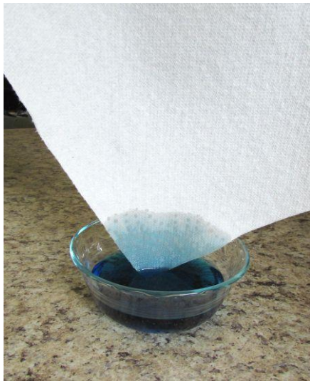
Figure 2.2 Capillarity in water
